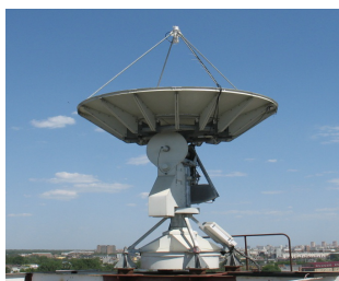
MEOLUT at new Russian monitoring station
