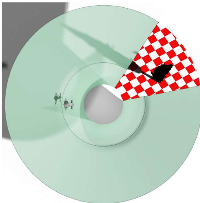
Figure VPT-B-20: Vertiport obstacle-free volume with omnidirectional approach and take-off climb surface and prohibited sector — top view
