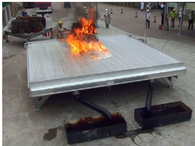
Figure II-6-6. A fire test on a passive fire-retarding surface (200 L of burning fuel)
