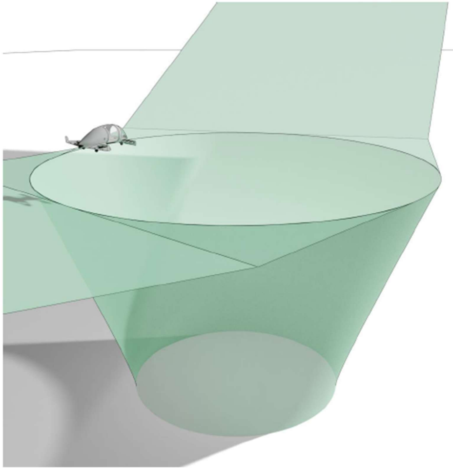
Figure VPT-B-17: Vertiport omnidirectional obstacle-free volume with discrete planar approach and take-off climb surfaces — perspective view
