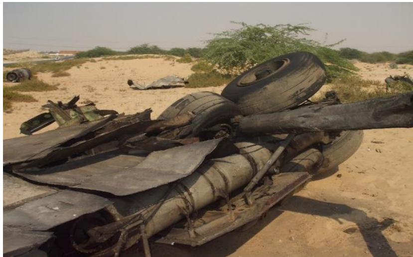
Figure 5. Pressurized tire as found at the accident site
