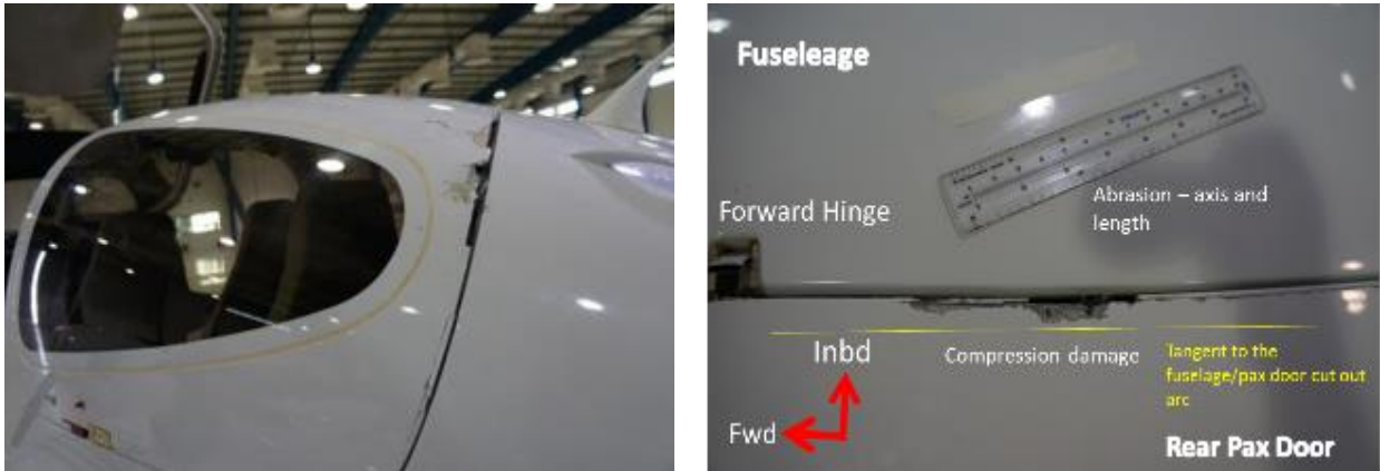
Figure 1. Passenger door damage
