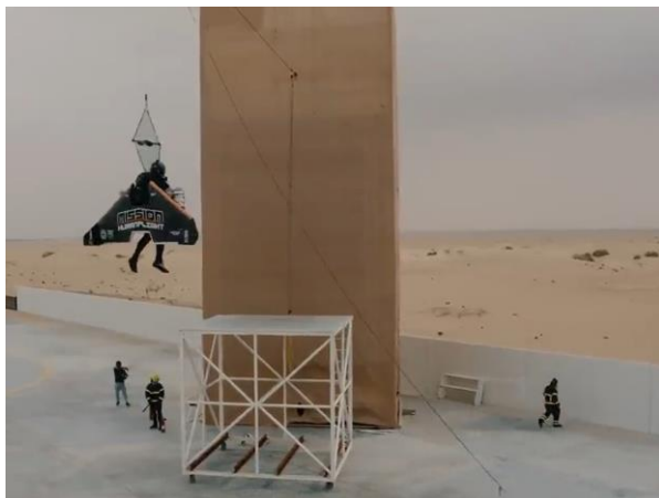
Figure 5. Tethered hover test [Source: Jetman Dubai]
