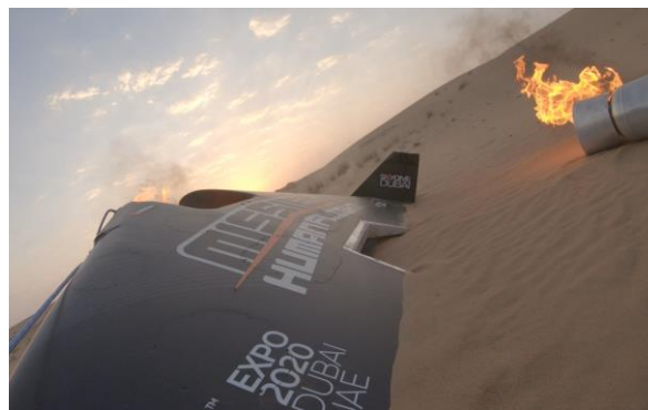
Figure 6. Jetwing fire after impact
