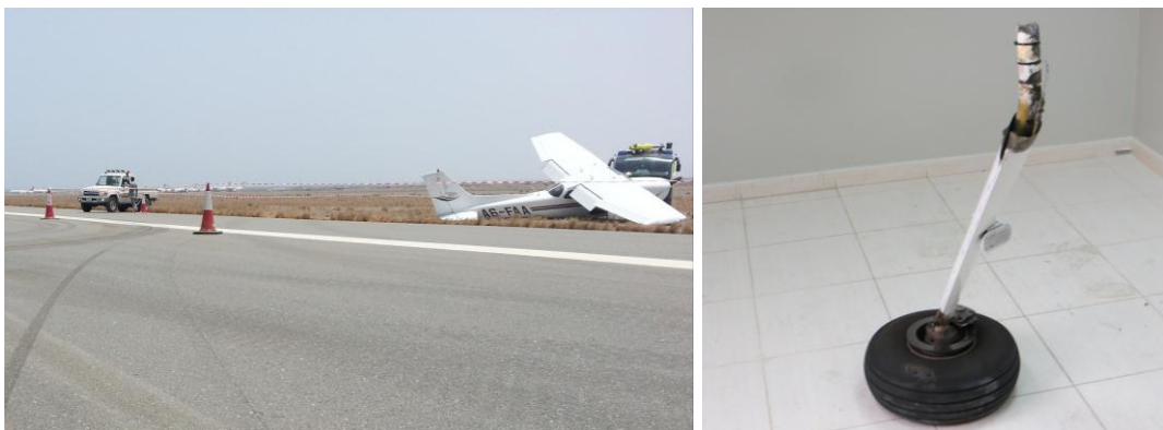
Figure 1. Runway excursion and RH Landing Gear Strut and Wheel Assembly
