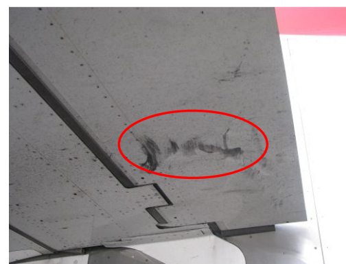
Figure 7- Lower surface of the L/H INBD flap shows a mark of the rubber chunk hit at high speed.
