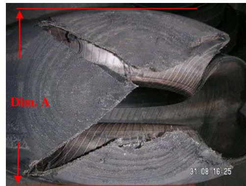
Figure 5- This portion of the tyre is the surface which made friction and caused the tyre skid mark (Dim. A in figure 3).
