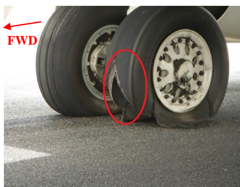
Figure 6- the place of a dismantled chunk that hit the L/H INBD flap lower surface (see figure 6 to the right).
