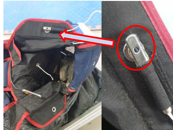
Figure 13. AAD cutter in the fatally injured Skydiver Parachute Container
