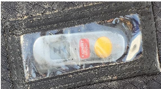
Figure 12. AAD status display- 'Standard Mode'
