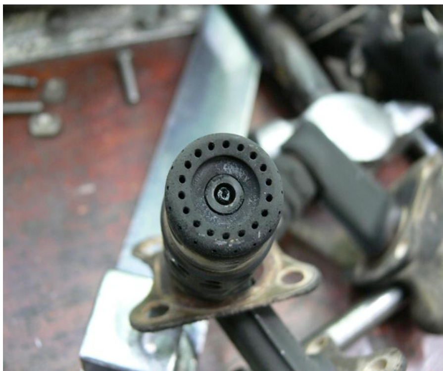
Figure 2- the most affected fuel nozzle
