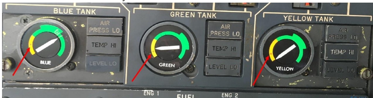
Figure 6. The Aircraft's hydraulic system indications after collision with the tug
