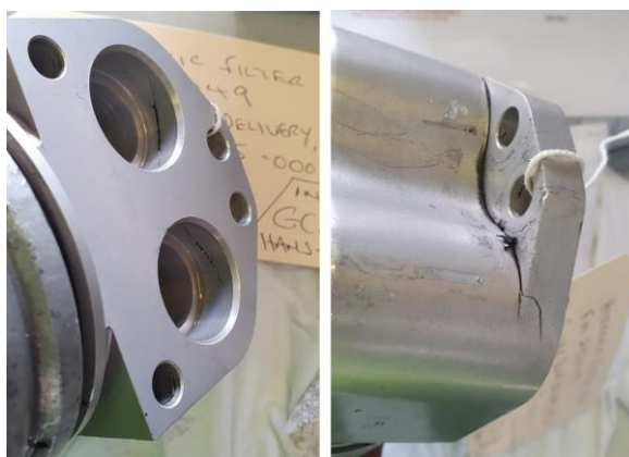
Figure 8. Hydraulic filter housing fracture
