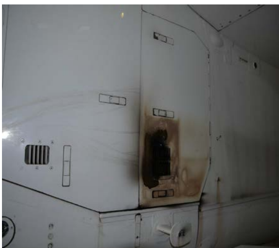
FIG 6 #2 Engine LH side access panel 425AL showing discoloration
