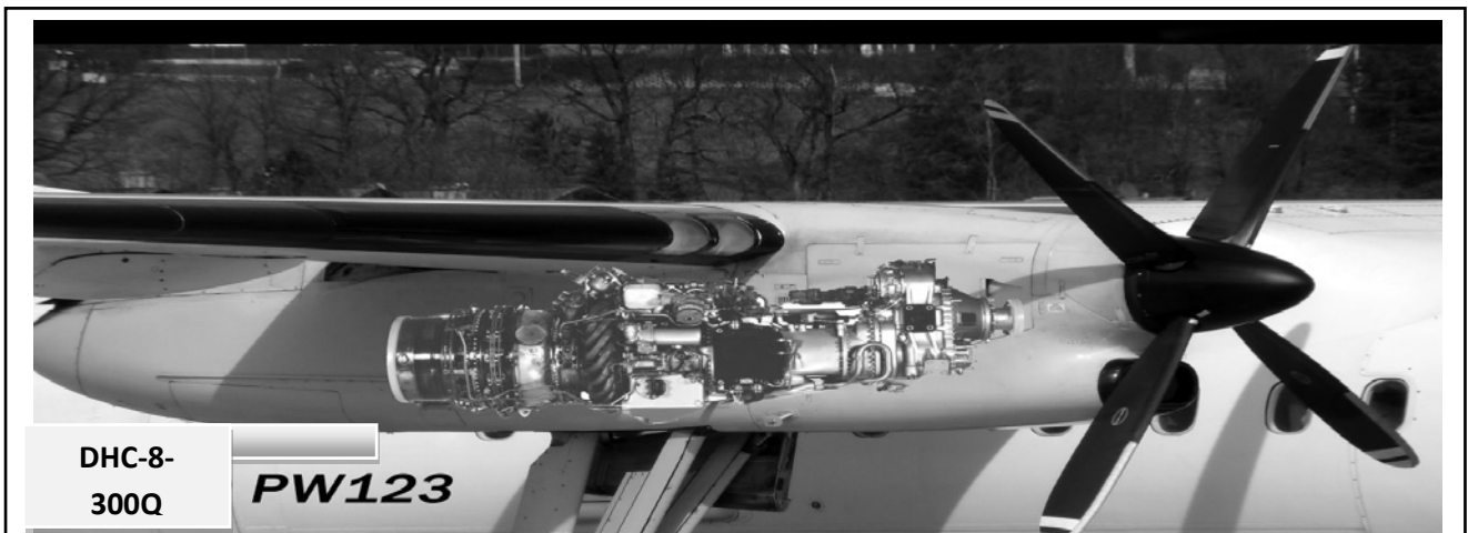
FIG 16 DHC-8-300Q showing the PW123 Engine and Propeller
