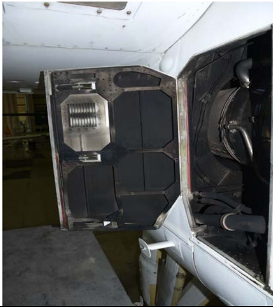
FIG 12 #2 Eng- RH side- showing signs of soot deposit
