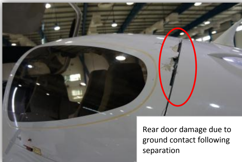
Picture 2 Damaged Door Reinstalled Fit Check
