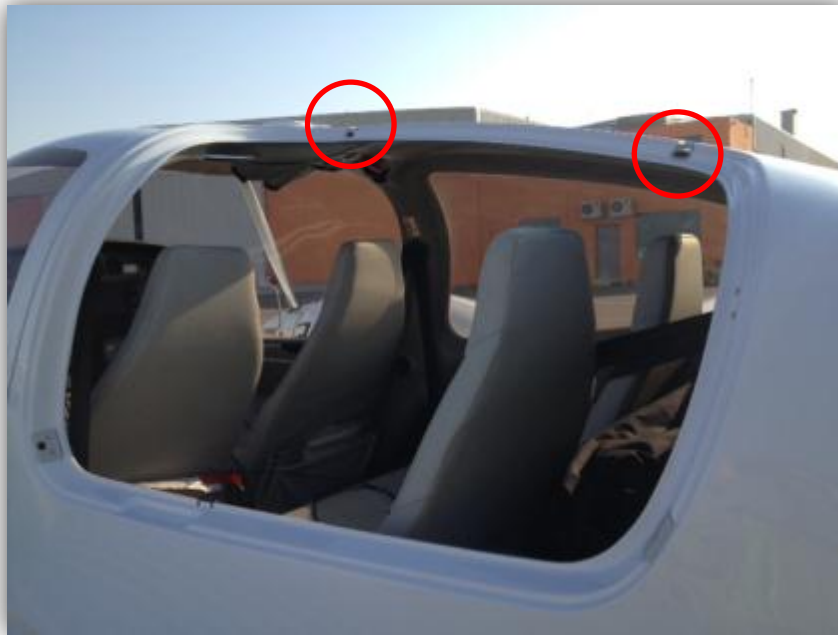
Picture 1 Door Hinge Location
