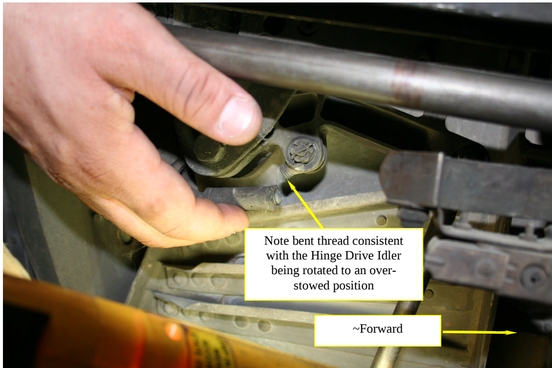
Photo (3) – Lower Left Adjustment Link Fracture
