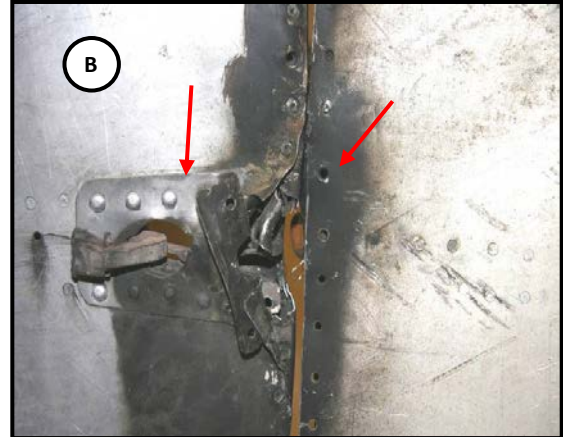
Example of skin repair around E latch assembly on the RH cowl and missing rivets on the LH cowl
