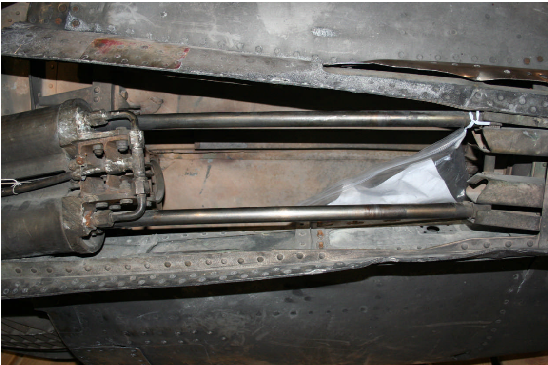
Photo (12) – Upper Actuator Rods
