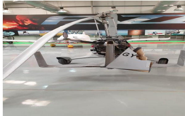
Figure 4. Damage to the tail
