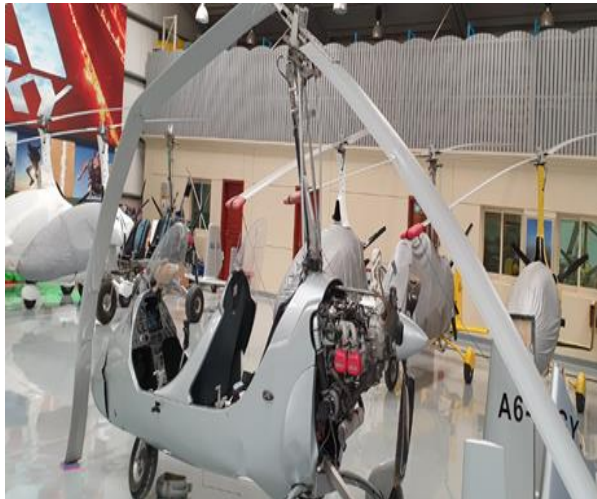
Figure 2. Damage to rotary blades
