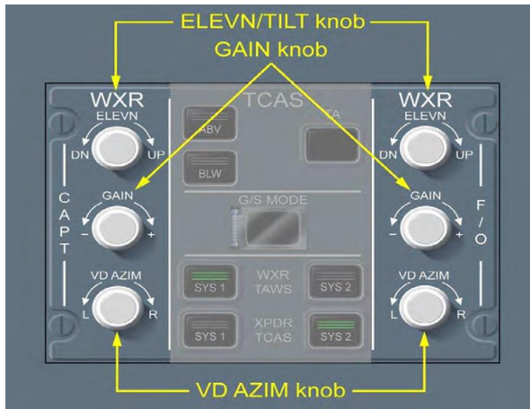
Figure 6. Weather radar rotating knobs [Source: FCOM-Surveillance Panel]
