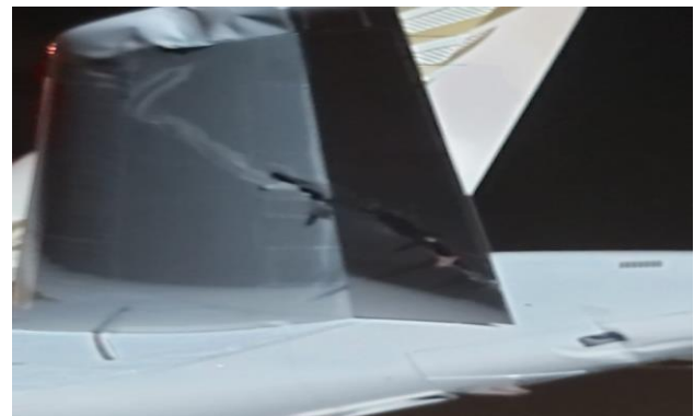
Figure 2. Damage to the A321 tail
