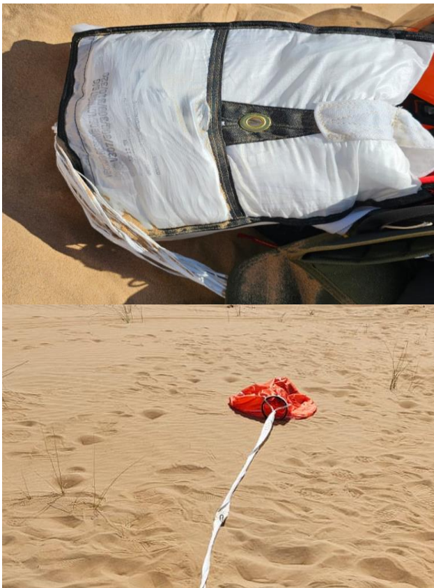
Figure 7. Pilot chute, main and reserve canopies
