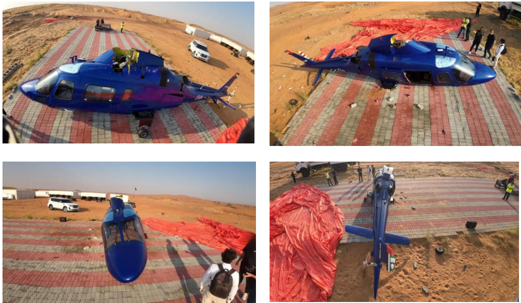
Figure 1. Helicopter damage and wreckage distribution
