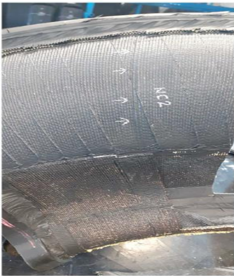
Figure 13. Joint on NC2 carcass
