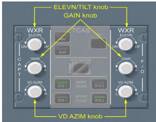
Figure 1. Weather radar rotating knobs [Source: FCOM-Surveillance Panel]
