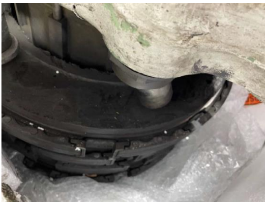
Figure 4. Damaged pressure plate and piston [Source: Collins Aerospace]
