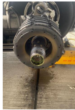
Figure 1. Hydraulic fluid leakage
