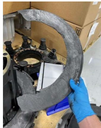
Figure 6. The remaining section of stator 2 [Source: Collins Aerospace]
