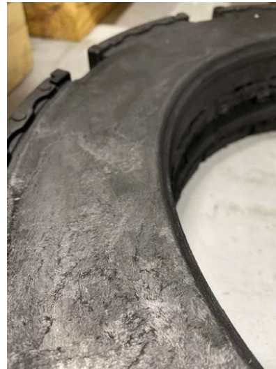
Figure 5. Damaged rotor due to contact with stator clips [Source: Collins Aerospace]
