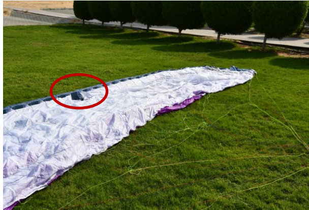
Figure 5. Damage at the leading edge of the wing
