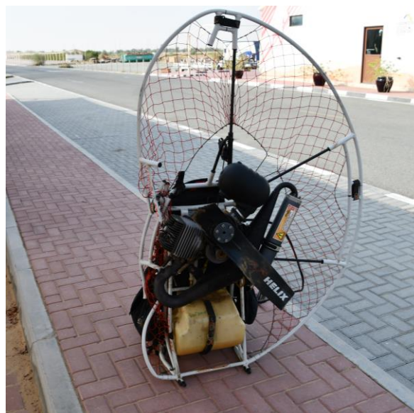
Figure 4. Damage to propeller's blades and cage
