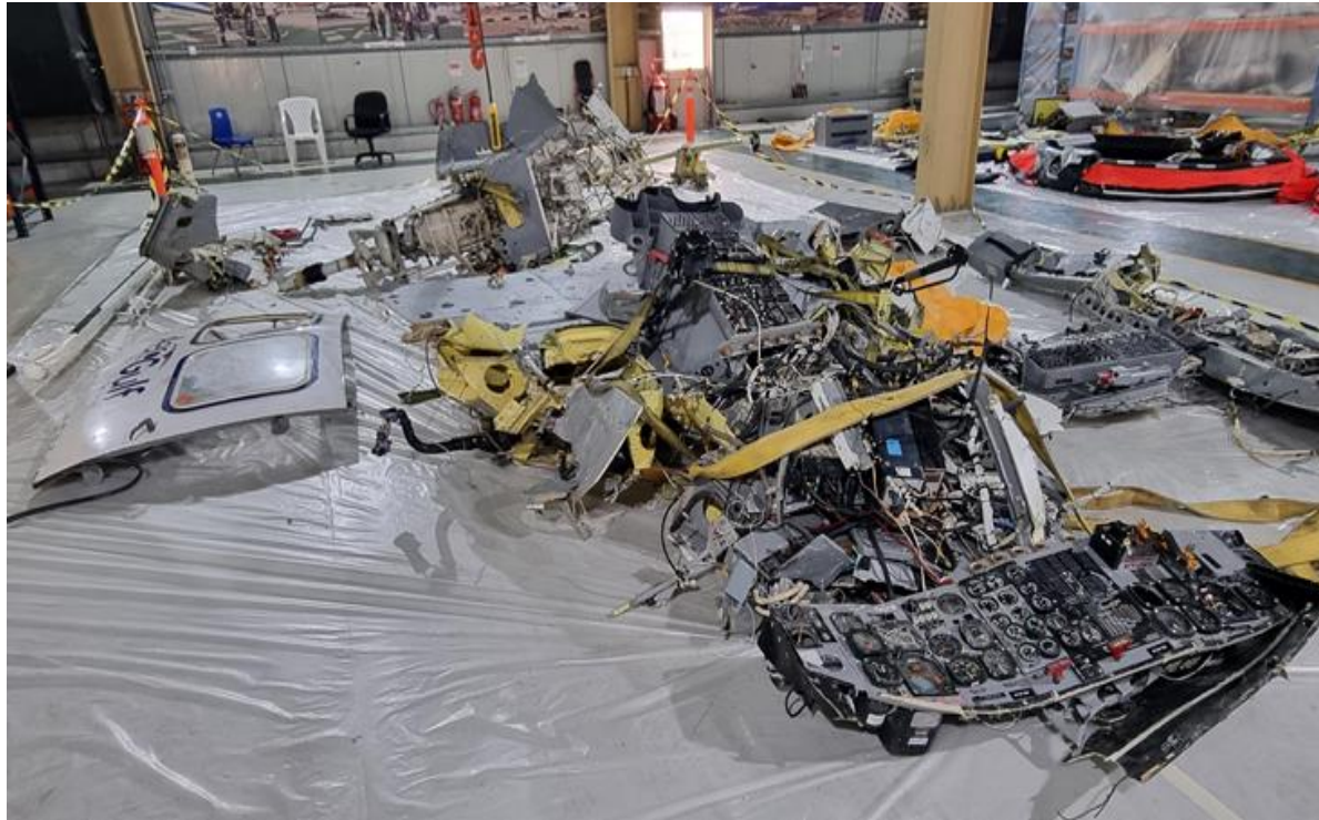
Figure 3. Wreckage recovered (cockpit and main transmission gear)
