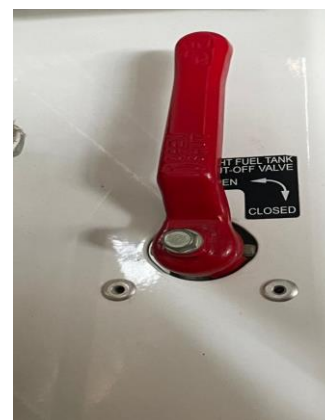
Figure 5. Fuel shutoff valve - Open position
