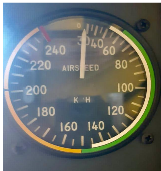
Figure 3. Airspeed Indicator (speeds in kilometers)
