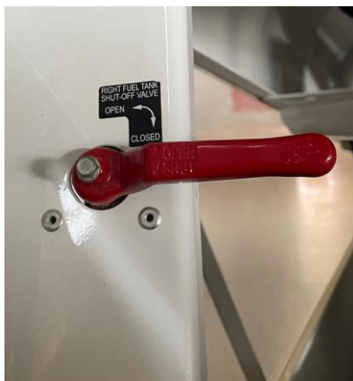
Figure 6. Fuel Shutoff valve - Closed position
