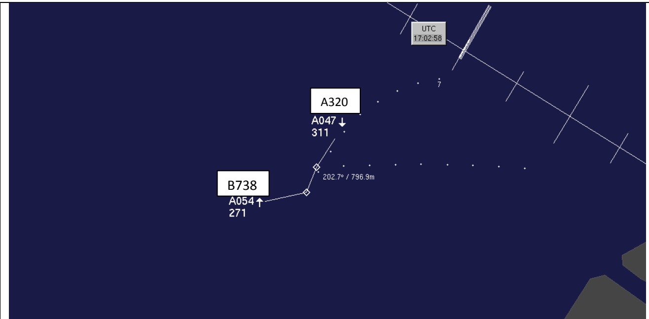
FIG 3. The A320 passes behind the B738. Vertical displacement = 700ft, lateral displacement = 2614ft.
