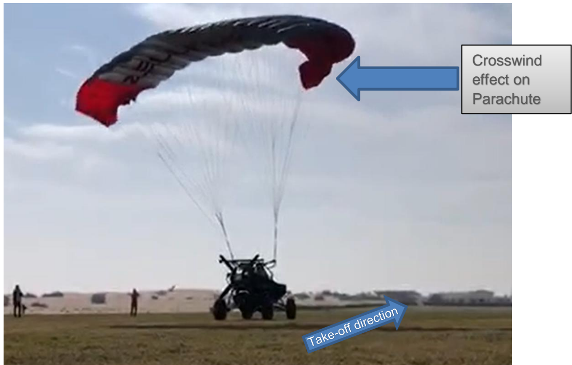
Figure 17. Crosswind effect on the parachute at the start of the takeoff roll
