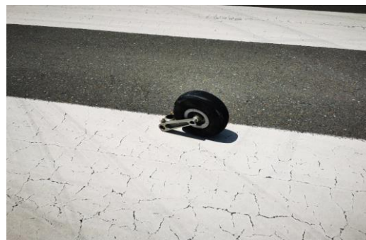
Figure 2. Detached nose gear
