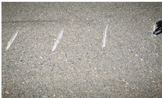
Figure 4. Slashes left by the propeller on the runway
