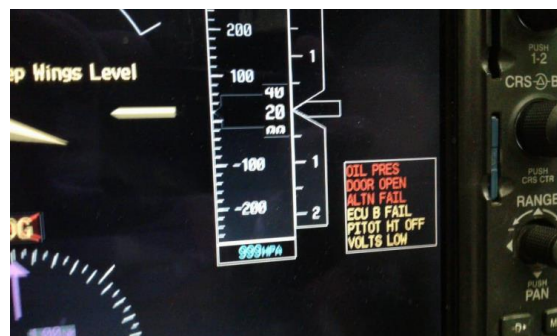
Figure 6. ECU B failure caution
