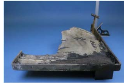
Figure 22. L1 cabin crew seat pan and left lever distortion [Source: NTSB]
