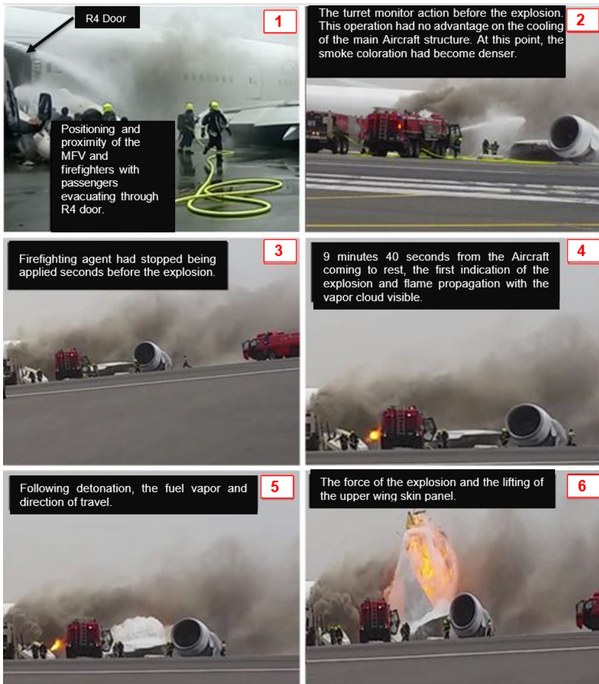
Figure 17. Center wing fuel tank explosion
