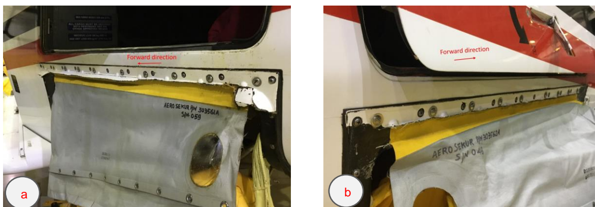
Figure 15. Left and right aft composite cover damage
