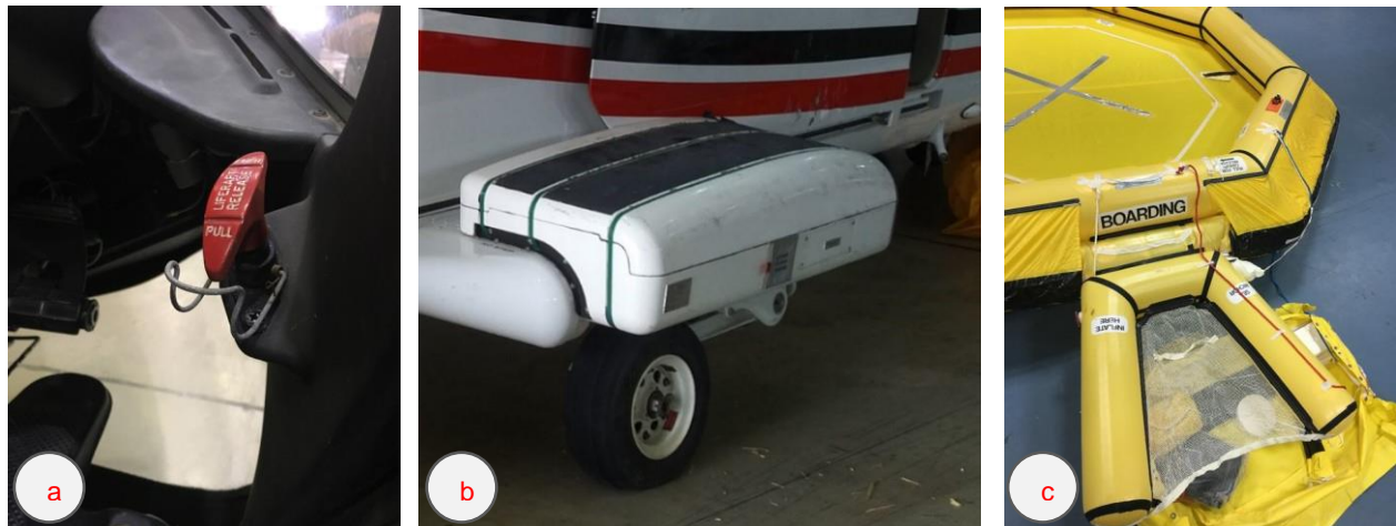
Figure 6. Raft deployment handle, raft sponson location and deployed raft assembly
