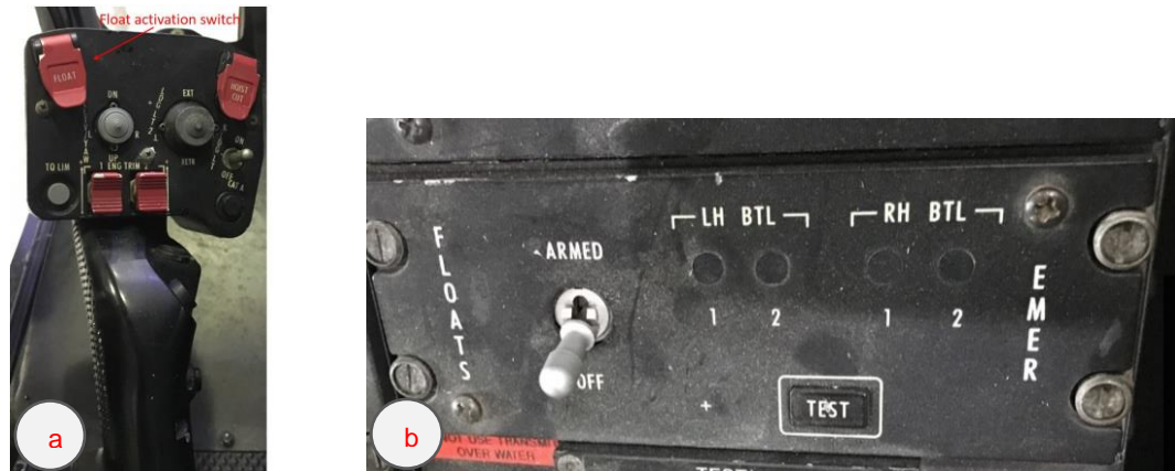
Figure 13. Flotation system activation switch and arming/test panel
