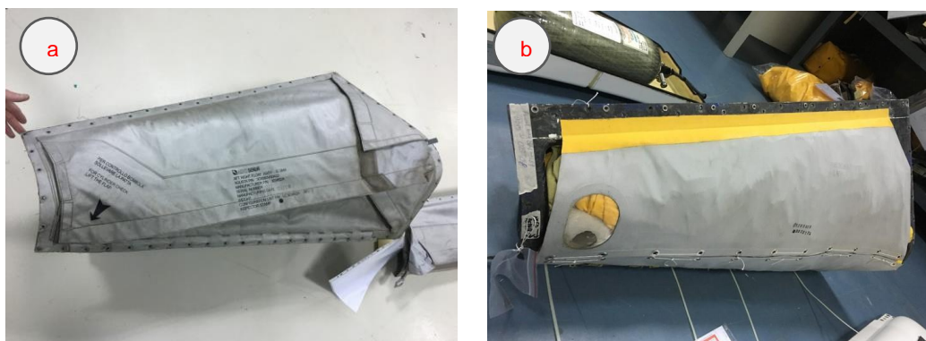
Figure 1. Textile flotation system and rigid system (rigid cover omitted)
