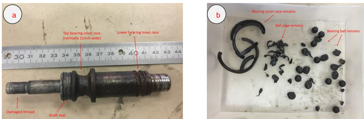
Figure 17. Cooling fan assembly shaft and bearing parts findings [Source: Leonardo Helicopters]
